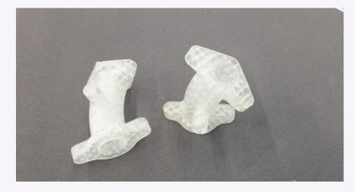
RR355-101-CASis a Direct casting material that was formulated for our Raplas production equipment. RR355-101-CAS offers the best performance characteristics as follows: low deformation due to shrink, strength, durability, water resistance. The RR355-101-CAS is transparent in colour.
